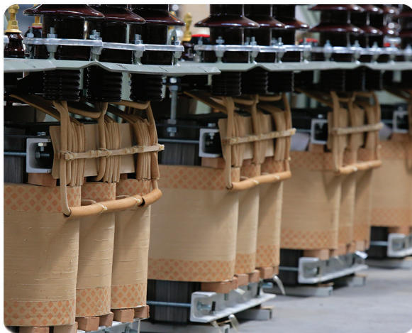
*Star diagram 20-30kV 10-30-63A 3-7 positions Setting 2.5 % per position
