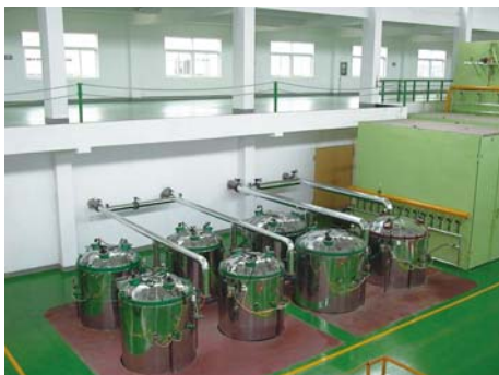
Vacuum Drying Clave for Condenser core
