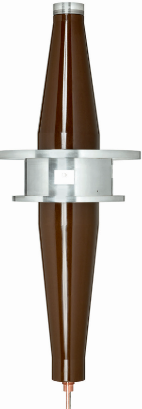
RIP/RIS technology • 72,5 – 550 kV • Up to 3.150 A
