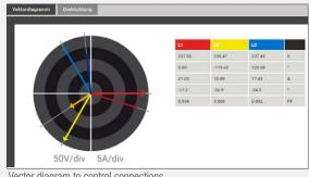
Vector diagram to control connections
