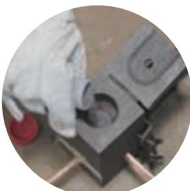
4. Pour weld metal powder into the mould cup.
