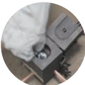
3. Place the steel retaining disc in the mould cup over the tap hole.
