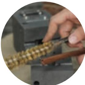
1. Conductors must be clean & dry when placed in the mould.
