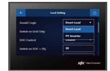
AC Out 2 for intelligent load control
